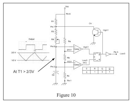
previous setting which was  $\underline{Q}$  low. The state of the transistor remains off meaning C2 will continue to charge, and the output on pin 3 also remains unchanged at high.
