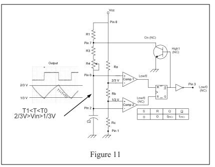
the previous state, the output on pin 3 is unchanged at low, and the transistor remains turned on to continue the discharge of C2. This state remains until the cycle is repeated at T0 when the voltage drops slightly below 1/3Vcc.
