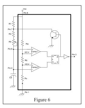
that is controlled by the output of the RS Flip-Flop that is connected to the base of the transistor.
