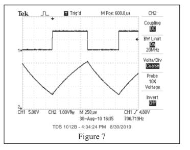
voltage rises above 1/3Vcc up to 2/3Vcc, the output flips high (Vcc) and remains high. As the input voltage rises just above 2/3Vcc, the output flops low or 0 volts. As the input voltage falls below 2/3Vcc down to just above 1/3Vcc, the output remains low. Finally, as the voltage falls just below 1/3Vcc and begins to rise again, the output flips to the high state to complete one cycle of oscillation. The rate of the input voltage change is
