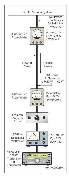
Figure 3 — This is the same situation as Figure 2, except that the antenna has an impedance of 12.5  $\Omega$ , a 4:1 SWR. Note that due to the loss in the transmission line going up to the antenna, and in the reflected signal coming back, it looks at the radio end as if the SWR is just 2.6:1. Even more confusing is the meter at the radio, showing 100 W out going to a perfectly matched system.
