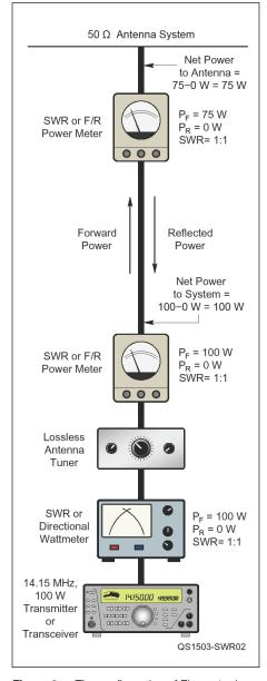
Figure 2 — The configuration of Figure 1, showing expanded instrumentation. While this would not typically be used, the numbers that would be obtained will assist in the discussion. For this example, we use 100 feet of the popular RG-8X coaxial cable to connect our radio to a perfectly matched antenna system on 14.15 MHz.
