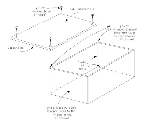
Figure 1—The oscillator sub-enclosure, fabricated from pieces of single-sided PC-board material.
