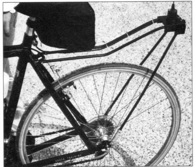
Fig 3—The vertical supports of the antenna mount serve as the resonant counterpoise.
