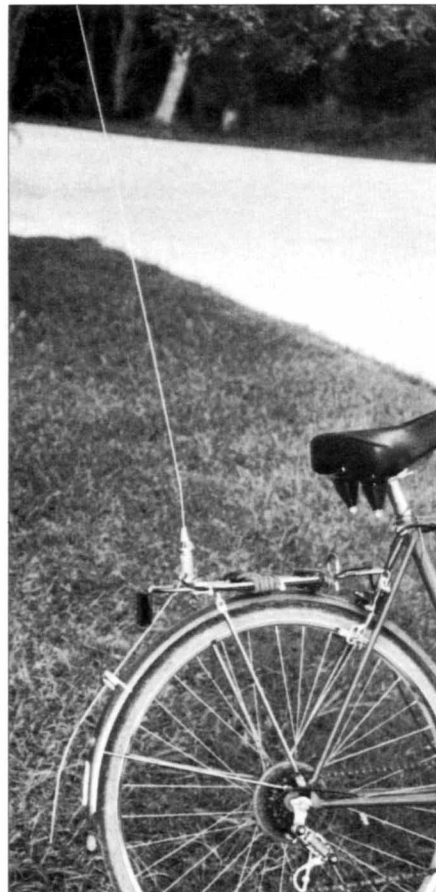
Fig 1—A \frac{5}{8} -wave antenna and counterpoise mounted on the back of a bicycle luggage rack. (photos by Steve Cerwin, WA5FRF)
