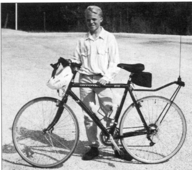
Fig 2—Andy Cerwin with his father's hybrid bicycle. The bicycle is equipped with a resonant antenna mount and \frac{5}{8} -wave antenna.
