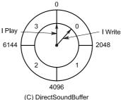
Fig 2—DirectSoundCaptureBuffer and DirectSoundBuffer circular buffer layout.
