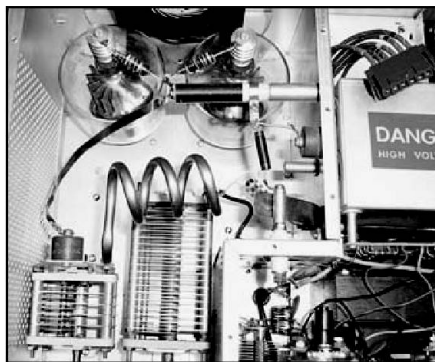
Figure 4 — New plate and input circuits. The original parasitic suppressors remain.
