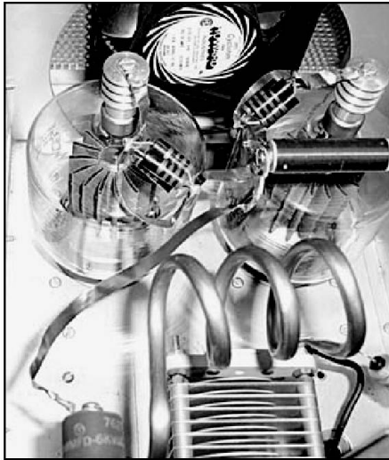
Figure 8 — Note the piece of Nichrome ribbon leading from RFC1 to doorknob capacitor C29.
