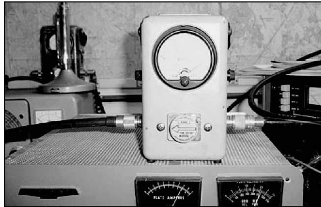
Figure 9 — Glare prevents a clear view of the Bird meter being buried on a 1 kW slug.
