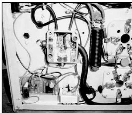
Figure 6 — Vacuum relays are in the die-cast box. The 12V power supply and bias relay are located below.
