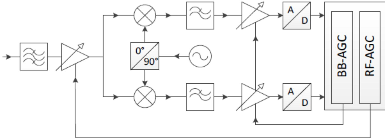
The broadband AGC serves to protect the AD converter from overvoltages. The RF-AGC can be used to set the receiver sensitivity just below the external noise.
