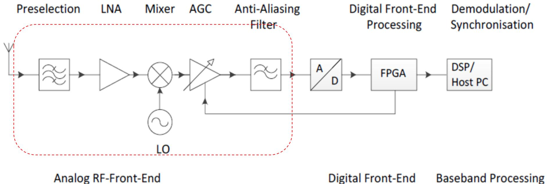
The analog front end is downconverting the RF signals into an IF range <200MHz
