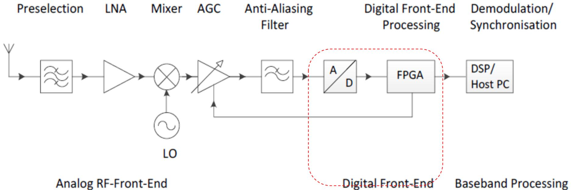
The digital front end consists of an Analog to Digital converter and a digital down- converter to reduce the sample rate down to the bandwidth needed by the application. Sampling rate of AD converters are rising up to 250Mpsps with resolutions of 14 or 16 bits.
