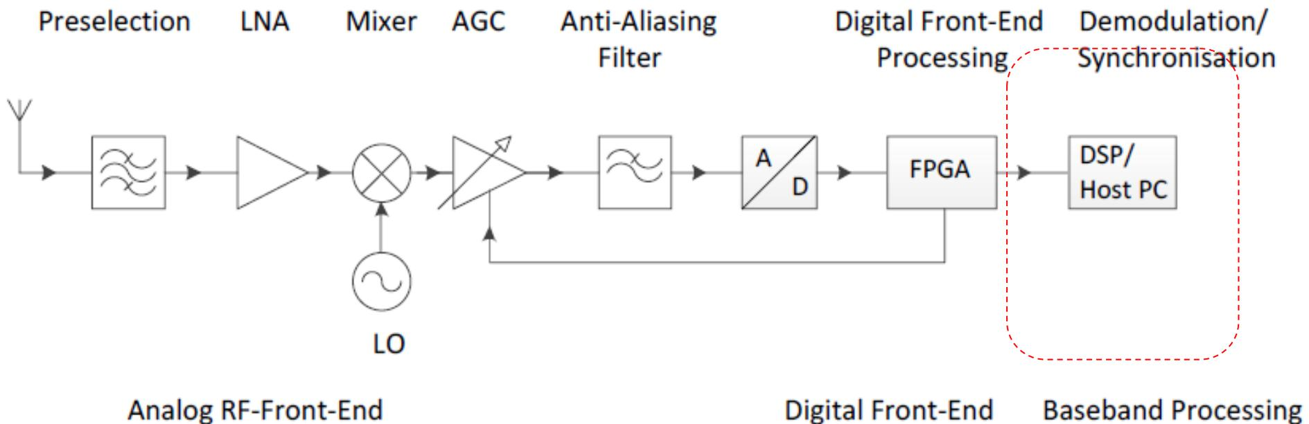
The baseband processing takes over the base band filtering, AGC, demodulation, and the signal regeneration..
