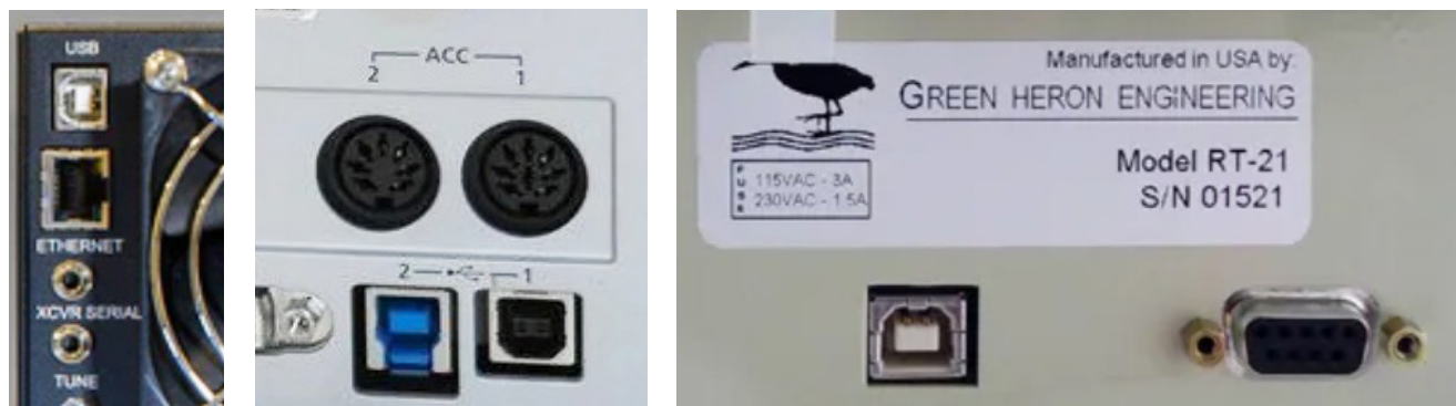
Figure 2 — The back of an Elecraft KPA1500, an Icom IC-7610, and a Green Heron RT-21 showing the USB-B port.
