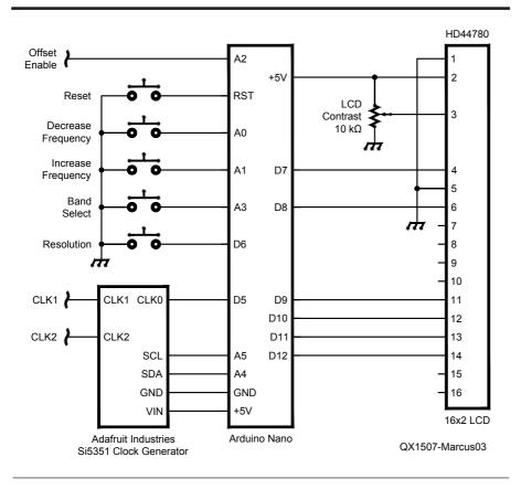
Figure 3 — This is the schematic diagram for the basic non-GPS configuration of the Si5351 VFO project. Either an Arduino Nano or Arduino Uno can be used.
