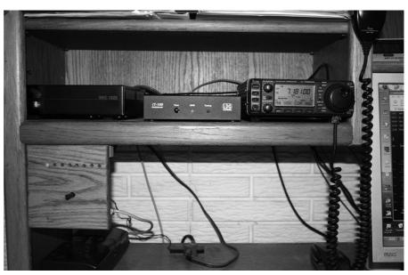
Figure 2 — This photo of my operating position shows my power supply, LDG Autotuner, and lcom IC-706 MKIIG radio. The antenna selector control panel is mounted behind a block of wood to match the operating position shelf. You can see the selector shaft, with the first of eight LEDs illuminated to show which antenna has been selected. I still have to add labels below the LEDs to help identify the antennas.
