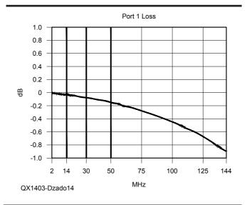
Figure 14 — This graph shows the signal response (S<sub>11</sub> parameter) versus frequency for port 1. The responses for the other ports are virtually identical.
