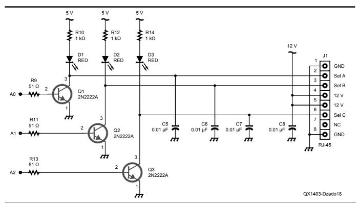
Figure 18 — This schematic diagram shows the remote control wiring output to the antenna selector switch.
