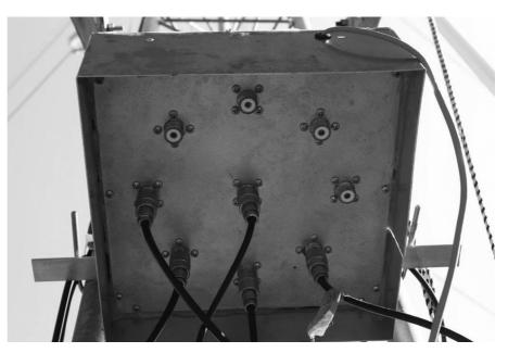
Figure 1 — The remote antenna selector board is mounted on the side of my tower. As shown here, it is selecting between four antennas.
