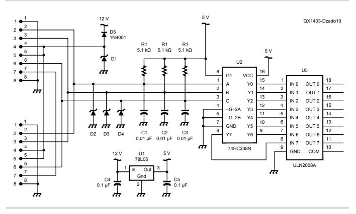
Figure 10 — The schematic of the antenna selector control logic. U2 is a 74HC238 3-to-8 decoder IC and U3 is a ULM2008A high current, 8 pair Darlington transistor array to provide the relay drive current.
