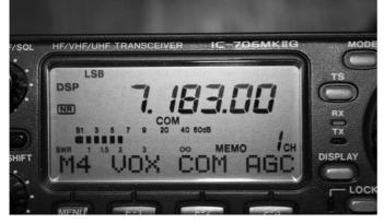
Figure 3 — Here is a close-up of the Icom radio display. Notice that with a 40 m antenna connected, the S meter is showing an S6 signal.
