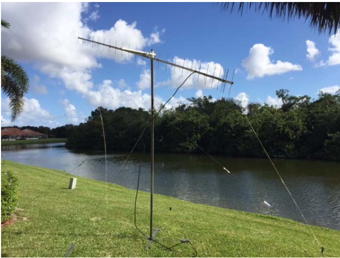
A single, vertically-polarized 70 cm Yagi at the K1DS winter QTH in EL96 (Florida). (Photo – credit K1DS)
