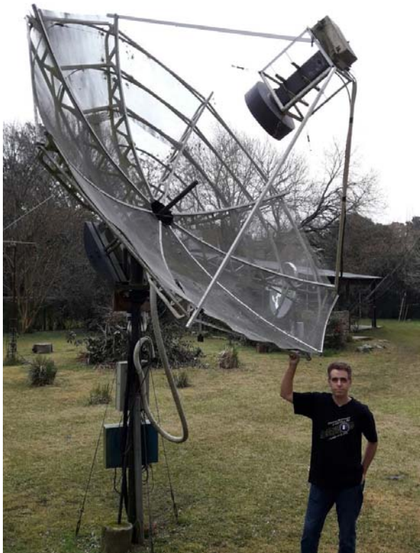
Juan LU9DO of the LU1CGB multioperator team on VHF JT65 with 4 Yagis, and 600 watts. In the bottom photo Adrian, LU1CGB shows off the 3.6-meter dish used on 23 cm with an RA3AQ feed and 250 watts. (Photo – credit LU1CGB)
