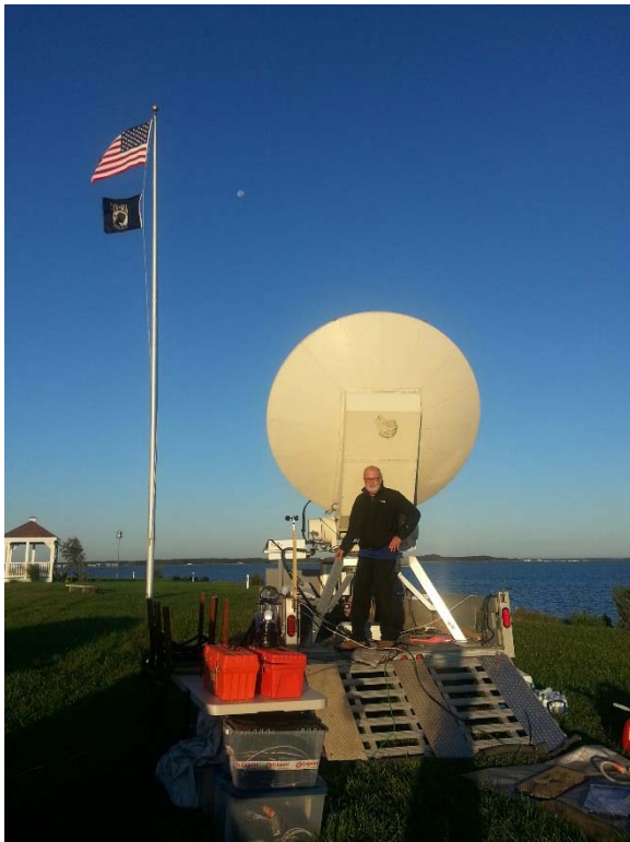
Jim, WA3LBI on the Delaware waterfront with his 2.4-meter trailer-mounted 10 GHz station. He and Rex, VK7MO set a new 10 GHz distance world record during the contest. (Photo – credit N2EME)
