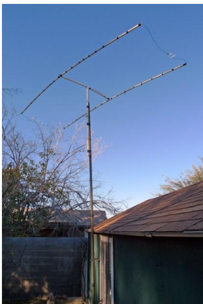
Figure 12 — Andy managed 248 QSOs and 98 multipliers with this homebrew Moxon beam (Photo – NY7N)
