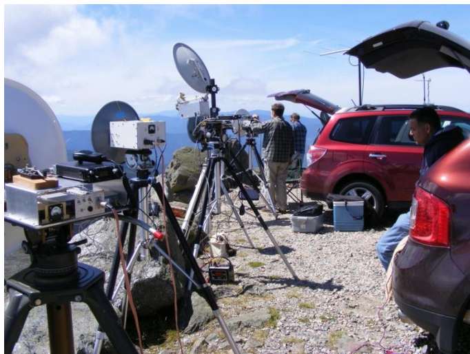
Mt. Washington (FN44ig) on the August weekend. Left to right are W1EX 10 GHz, W1EX 24 GHz, W1FKF 10/24 GHz, W1FKF spare 24 GHz, N1JEZ 24/47 GHz (hidden), N1JEZ 10 GHz, W1AIM 10 GHz, and K1LPS 10 GHz. (Photo N1JEZ)
