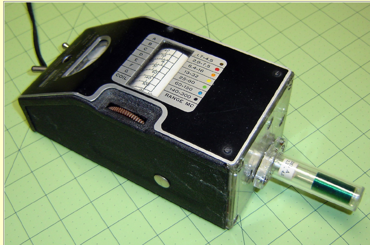
This Millen dip meter, also known as a "dipper", has the plastic plug-in coil for 80/75 meters installed at the rear. The tuning thumb wheel is on top of the housing next to the analog frequency readout display. There are two toggle switches on the front face which turn on the 110 volt power and the filament voltage to the unit.
