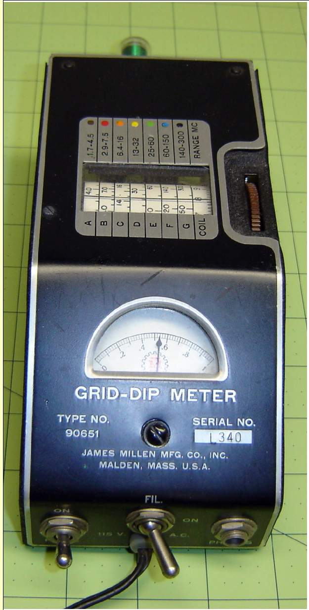
This is the front panel of the Millen Dip Meter with the unit powered up. There is an earphone jack on the right front of the panel where you could listen to "beat" frequencies of signals from the circuit under test. Before the advent of high accuracy frequency counters this was another way for determining the frequency of the signal.
